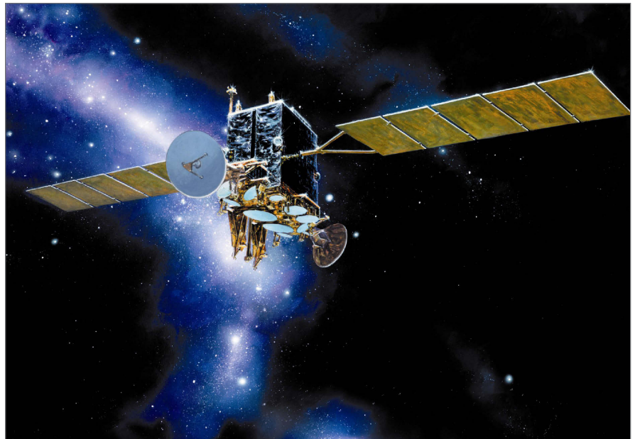
Figure 2 | One Advanced Extremely High Frequency (AEHF) satellite will provide greater total capacity than the entire Milstar constellation currently on orbit. Photo courtesy of Northrop Grumman.
