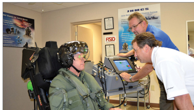
Rockwell Collins employees Dan Kalsow (back) and Rodney Breuer (front) test to ensure a pilot's pupils are within two millimeters of exact center to be properly aligned with the optics package on the F-35 HMDS. (Photo courtesy of Rockwell Collins.)
